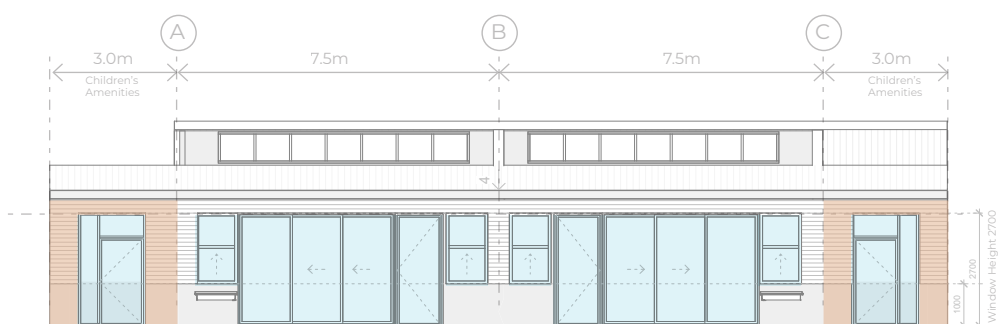
Concept Playroom Facade-North Elevation (40 Module)
